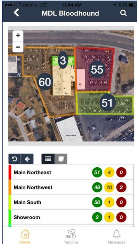
All employees at the store that are responsible for moving/finding vehicles use MDL's mobile and desktop applications to locate the inventory to within a 4-6 car radius. The solution was designed to be low cost without the need for complete support infrastructure with location updates performed by anyone walking in proximity to a vehicle.
